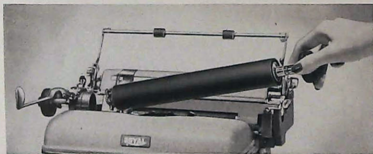
Removing the cylinder of the Royal is a simple motion requiring but two fingers.
